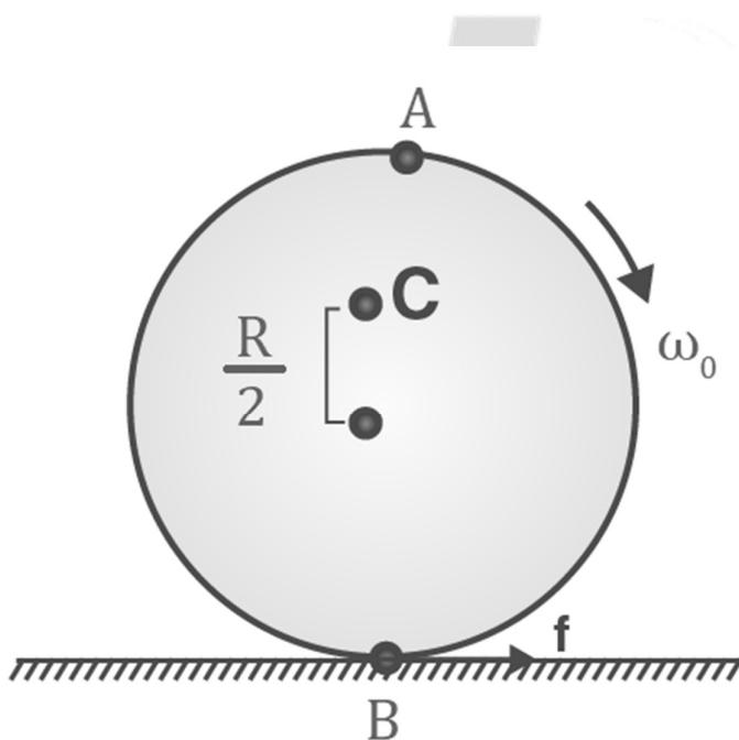
(a) The frictional force acting on the disc must be opposite to the direction of velocity. The frictional force acts towards the left as it opposes the direction of velocity at point B, which is towards the right.
